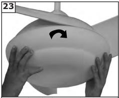
Attach glass by locating dimples in light fixture with the groves in glass and twisting clockwise till tight.
